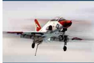
The pilot descends the aircraft to 600 feet and performs landing checks (e.g., flaps, landing gear, tail hook) prior to Base Leg, in preparation for landing.
