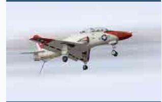
The pilot begins a gradual descent in a 180-degree approach turn, until intercepting the extended centerline of the carrier's landing area.
