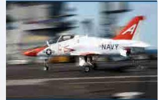
The aircraft tail hook catches the arresting wire upon landing.
