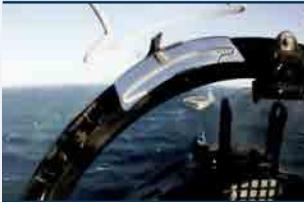
The pilot rolls the aircraft to wings level on the extended centerline to allow a 15- to 18-second groove before aircraft touchdown.
