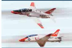
The pilot performs a 180-degree overhead turn at 800 feet to enter the landing pattern.
